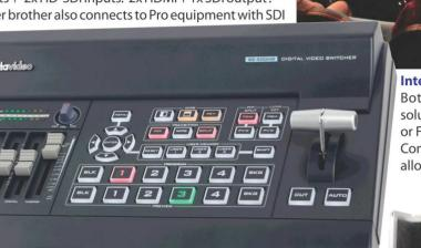
SE-500HD's features include Luma key for graphic overlay, SE-650's features add Chromakey and user assignable HD outputs as well as logo insertion. Both have split screen for podcast interviews, and PIP for Power point presentations. Microphones and other audio sources plug directly into the on-board audio mixer, and are embedded into the HD output.
